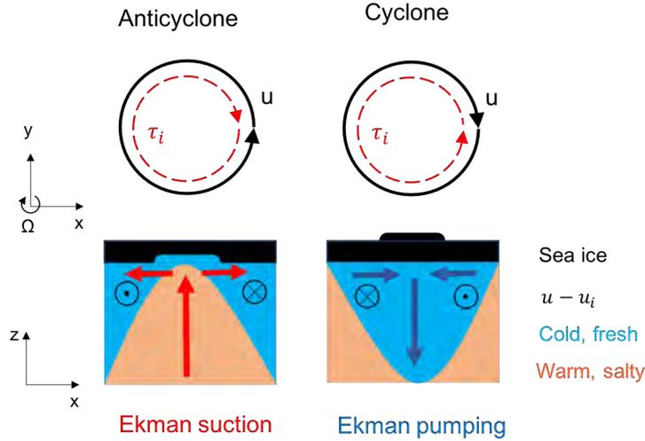
**Figure 1.** Schematic of the ‘Eddy-Ice-Pumping’ mechanism (EIP) in the Southern hemisphere. When sea-ice is stationary relative to the eddy, the ice-ocean stress  $\tau_i$  opposes the eddy motion  $u$ , driving Ekman suction in anticyclones and Ekman pumping in cyclones. Upwelling of warm waters may melt sea-ice in anticyclones, whereas downwelling in cyclones may shield sea-ice away from warm waters, potentially allowing for thicker ice growth.
